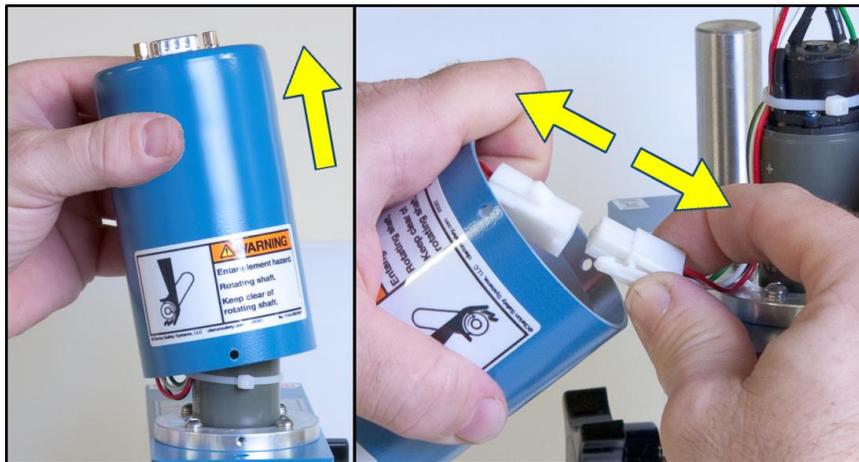
The internal cables are secured to the motor using two plastic cable ties.
