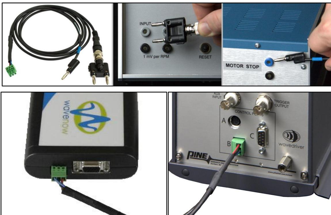
**Figure 4.15: Connecting the Rotation Rate Control Cable**
