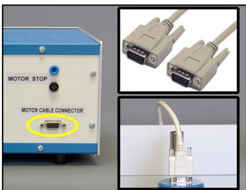
Remove the control unit **(10)** from the box and place it next to the enclosure base. Plug the male end of the motor control cable **(8)** into the motor cable connector on the back of the control unit, and plug the female end of the cable into the top of the motor unit.
