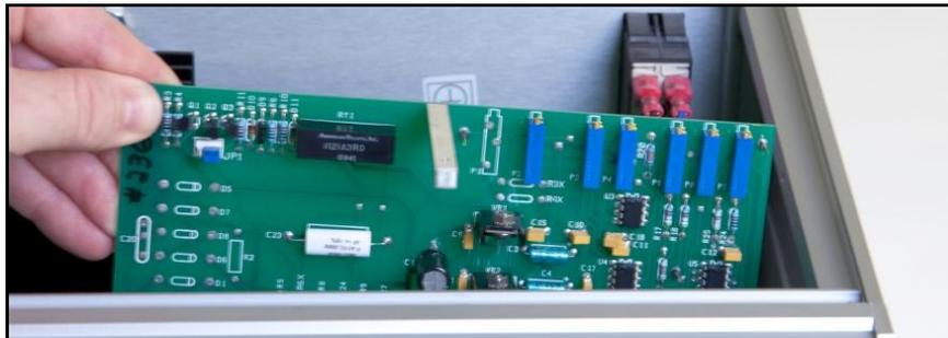
On the board, locate the configuration pins with the designation **JP2**. There is a small jumper that can be used to short together one of three pairs of pins.
