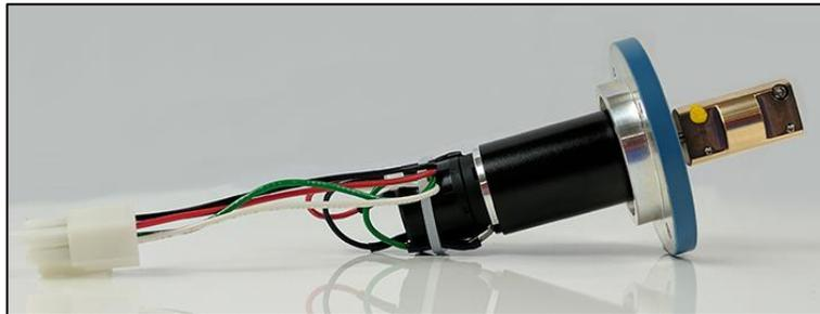
Remove any extra cable ties (i.e. around the green part of the motor) so that the cable can move freely.
