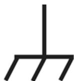
A **chassis terminal** is a connection to the metal chassis surrounding an instrument. Depending upon how the instrument is connected to other experimental apparatus, a chassis terminal may or may not be connected to the earth ground.
