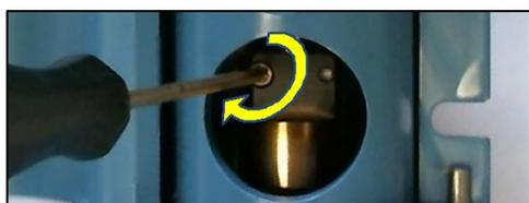
Use the hex driver tool (5/64") to securely tighten both hex screws on the motor coupling.
