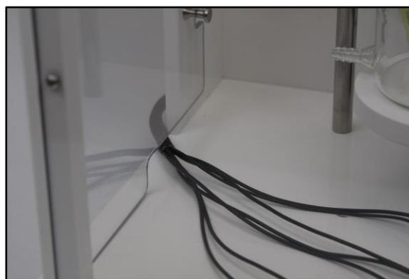
**Figure 4.11: Routing Cables out of the Enclosure**
