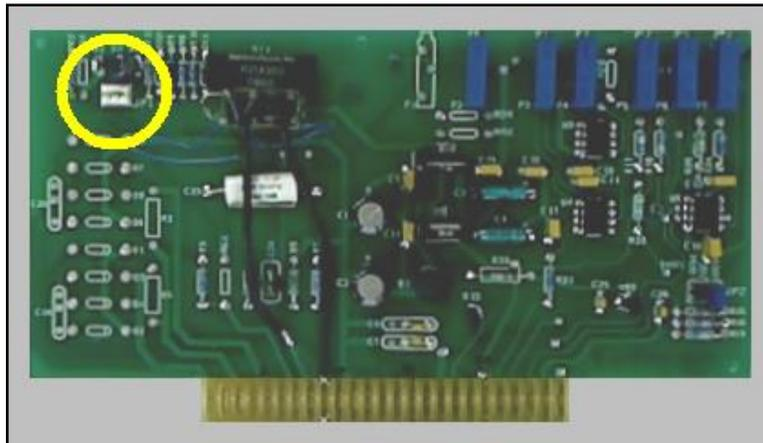
Place the jumper across one of the two positions shown below. Choose the position required for the particular potentiostat being used with the rotator.
