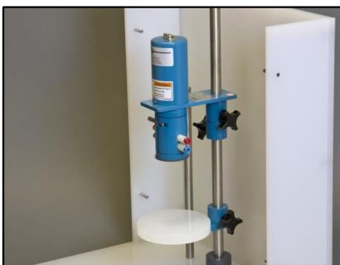
Carefully slide the motor unit **(2)** on to the center post **(1)** until it rests on the support collar **(5)**. Tighten the knob to secure the motor unit to the center post.
