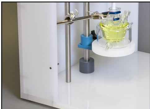
There are several holes in the floor of the enclosure base **(4)**, which are threaded to accept the side post **(6)**. Choose one of these holes and install the side post in it. Then, mount the laboratory clamp on to the side post.
