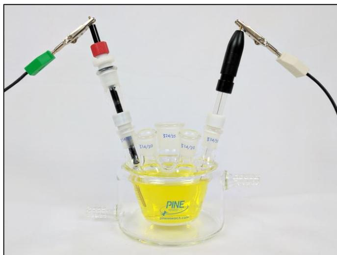
**Figure 4.7: Connection of Counter and Reference Electrodes**
