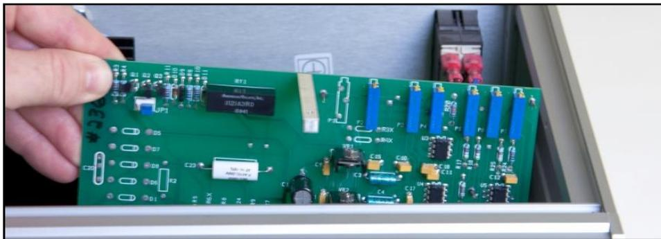
On the board, locate the configuration pins with the designation **JP1**. There is a small jumper that can be placed in one of two positions at this location.
