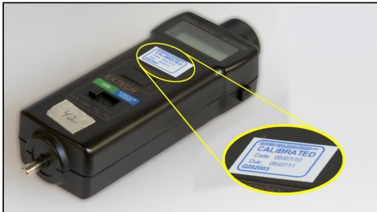
Figure 6.2: Professional Optical Tachometer with Traceable Calibration
