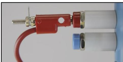
The upper (red) jacks make electrical contact with a rotating disk electrode (RDE) or a rotating cylinder electrode (RCE) tip.
