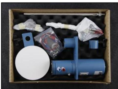
Open the smaller box. It should contain the motor unit (2), the support collar (5), the cell platform (3), the side post (6), a standard three-pronged laboratory clamp (with right-angle mount), and a small bag containing two banana cables and some additional assembly hardware.
