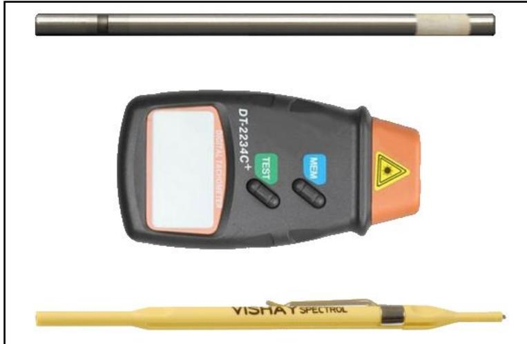
Figure 6.1: Rotator Calibration Toolkit (including simple handheld tachometer)
