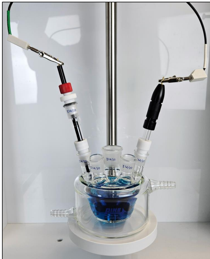
Figure 4-7. Connection of Counter and Reference Electrodes
