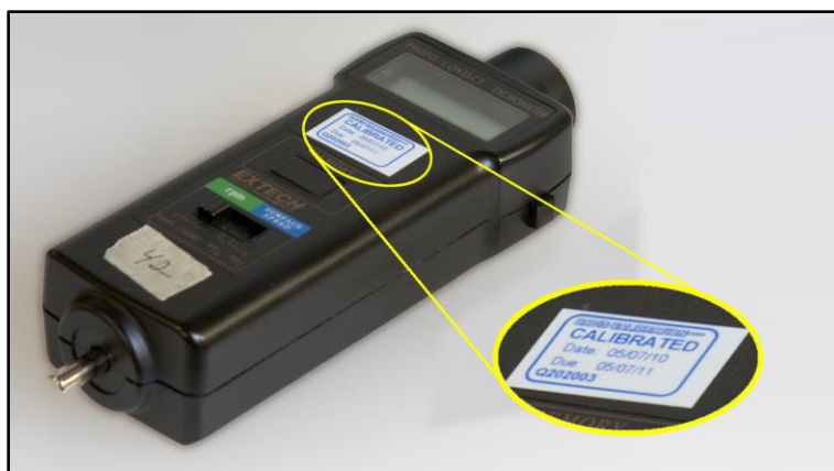
Figure 6-2. Professional Optical Tachometer with Traceable Calibration
