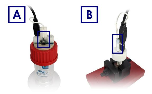
Figure 5-9. (A) Compact Voltammetry and (B) Spectroelectrochemistry Setups
