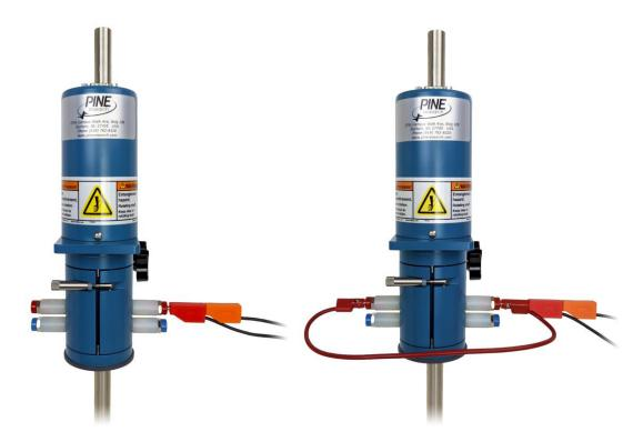
Figure 5-5. Working Electrode Connection for a Rotating Disk Electrode (RDE)
