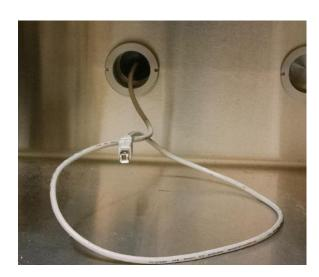
Figure 3-1. USB Cable Glovebox Feedthrough
