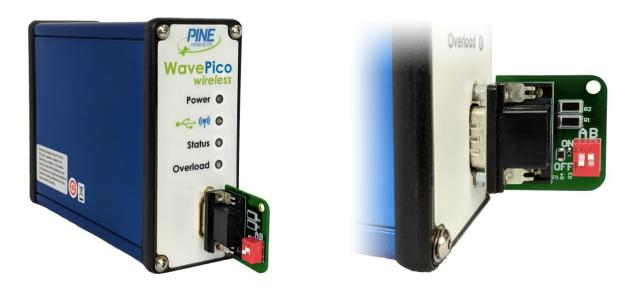
Figure 4-11. WavePico Wireless Connected to Dummy Cell with  $4.99~\text{M}\Omega$  Resistor Setting
