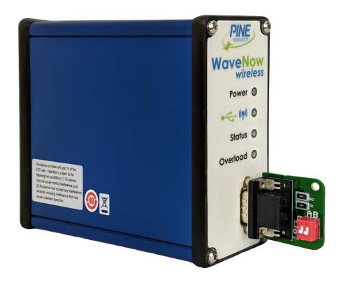
Figure 2-2. Dummy Cell Connected to WaveNow Wireless
