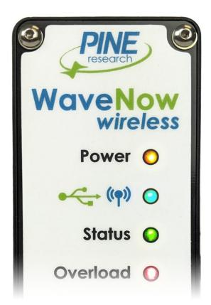
Figure 3-18. Instrument Light Status during Hardwired USB Connection (Blue-Green)
