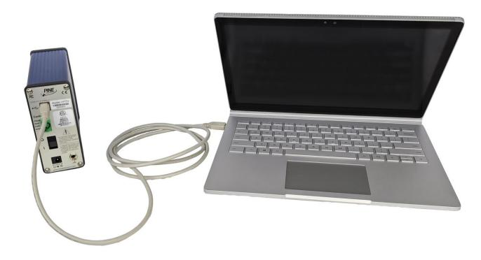
Figure 3-17. USB Cable Connection Between Potentiostat and Computer
