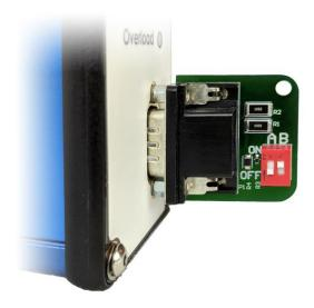
Figure 4-5. WaveNow Wireless Connected to Dummy Cell with  $49.9~\mathrm{k}\Omega$  Resistor Setting
