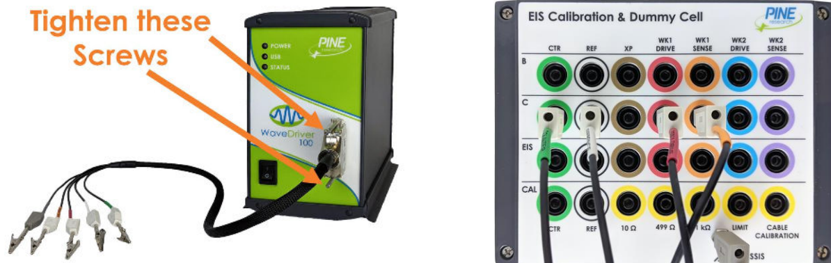
Figure 10-2. WaveDriver 100 Cell Cable Connected to Dummy Cell Row “C”
