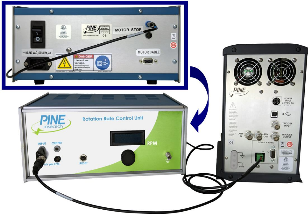
Figure 5-7. Rotation Rate Control Connections for a Pine Research MSR Rotator
