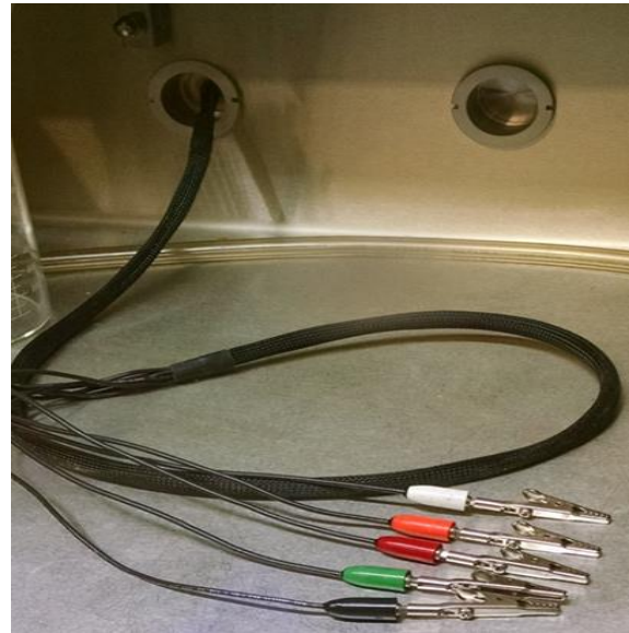
Figure 3-2. Cell Cable Glovebox Feedthrough
