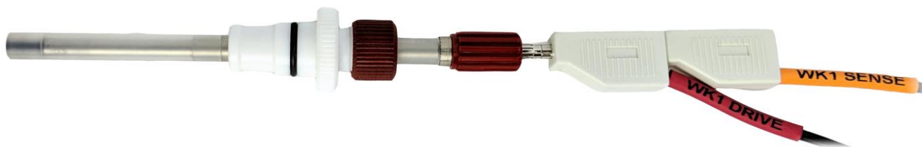
Figure 5-5. Working Electrode Sense and Drive Lines Shorted Together near the Electrode
