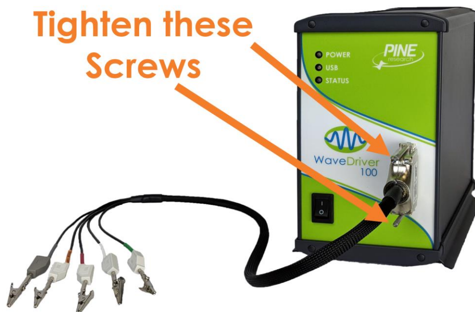
Figure 5-2. Secure Connection of the WaveDriver 100 Cell Cable to the Cell Port
