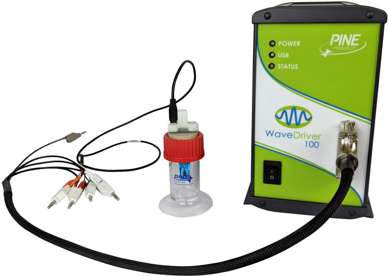
Figure 5-9. Cable Connections for the Compact Voltammetry Cell Kit
