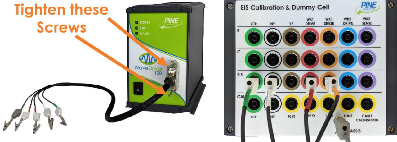
Figure 10-4. WaveDriver 100 Connections for a Simple EIS Test
