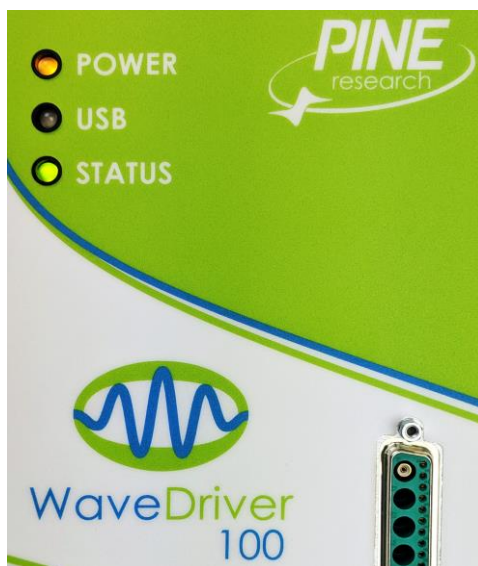
Figure 4-3. Indicator Lights on the Front Panel of the WaveDriver 100
