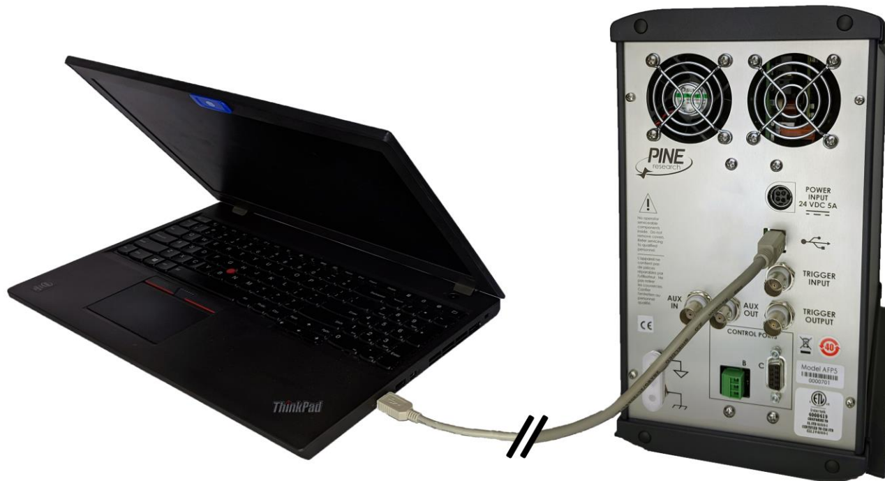
Figure 3-18. USB Cable Connection Between Potentiostat and Computer
