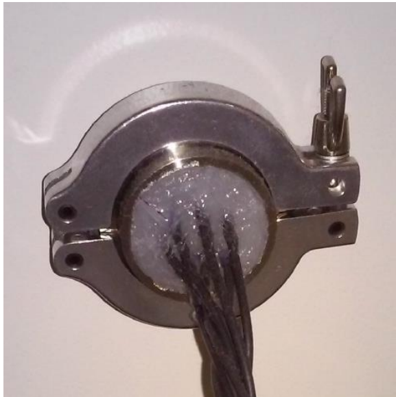
Figure 3-2. Cell Cable Glovebox Feedthrough
