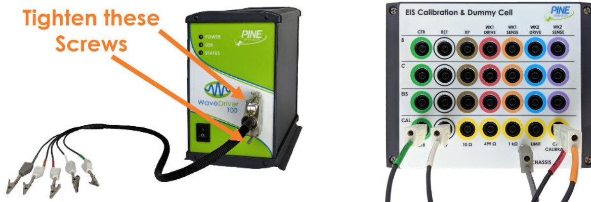
Figure 10-3. WaveDriver 100 Connections for Cell Cable Calibration
