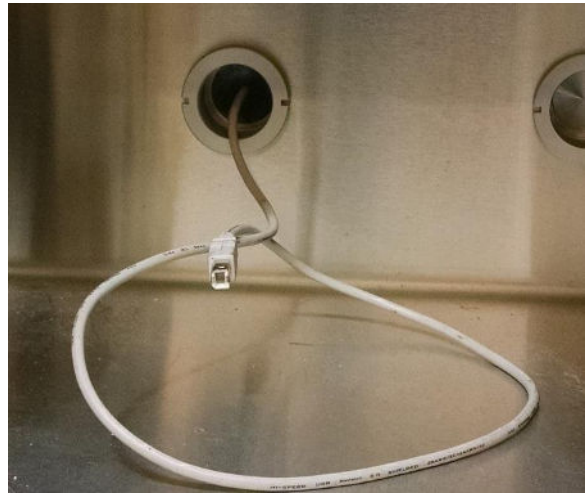
Figure 3-1. USB Cable Glovebox Feedthrough
