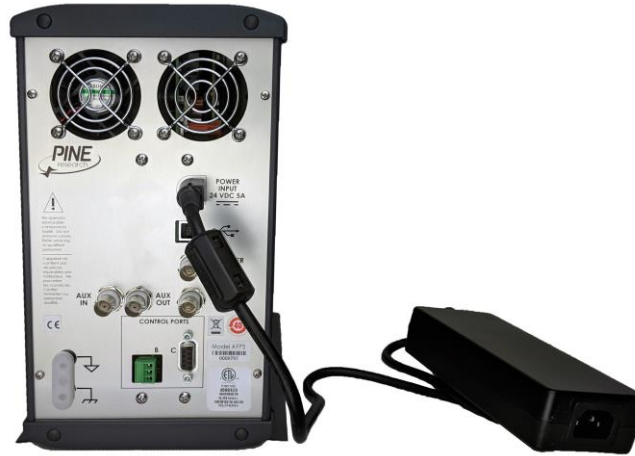
Figure 3-3. Power Supply with Low Voltage (24 VDC) Cable Connection to Back Panel
