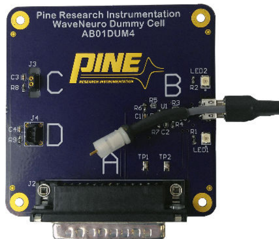
Figure 5-13. Connection of Headstage Cable to Dummy Cell B Connector
