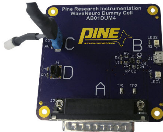
Figure 5-14. Connection of Headstage Cable to Dummy Cell C Connector
