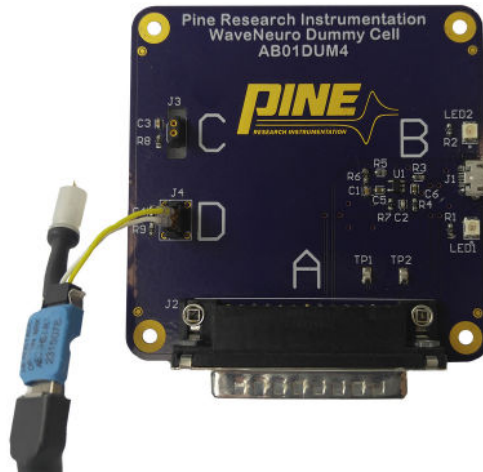
Figure 5-15: Connection of Headstage Cable to Dummy Cell D Connector
