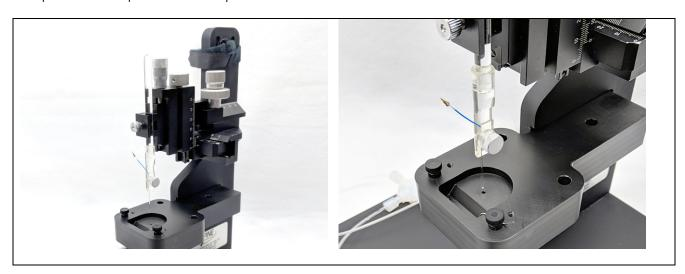
Figure 4-3. Installation of Microelectrode Holder into Micromanipulator
