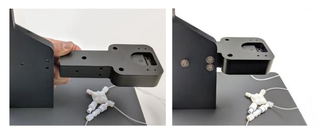
Figure 3-11. Attachment of Flow Cell Body to Arm
