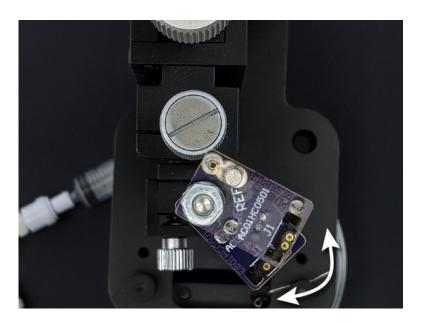
Figure 4-7. Malli Adapter for Flow Cell Variable Position
