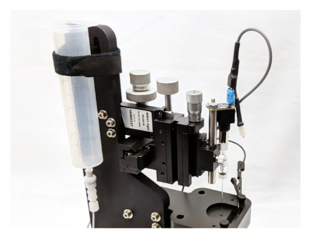
Figure 4-9. Fully Installed CFME in Using Malli Adapter in Micromanipulator
