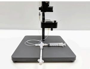
Figure 3-14. Completed Fluidic and Mechanical Assembly of Flow Cell
