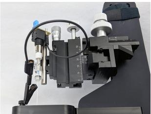
Figure 4-8. Connecting Electrodes to Potentiostat on a Malli Adapter for Flow Cell
