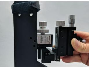
Figure 3-13. Attachment of the Micromanipulator to Arm
