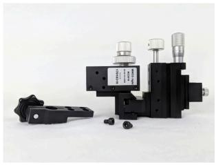
Figure 3-12. Removal of Micromanipulator Bracket
