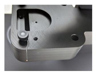
Figure 2-5. External Lead Thumb Screw Securing Reference Electrode Lead
