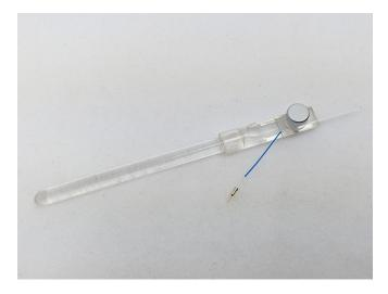
Figure 4-2. Installation of Microelectrode into Micromanipulator Electrode Holder
