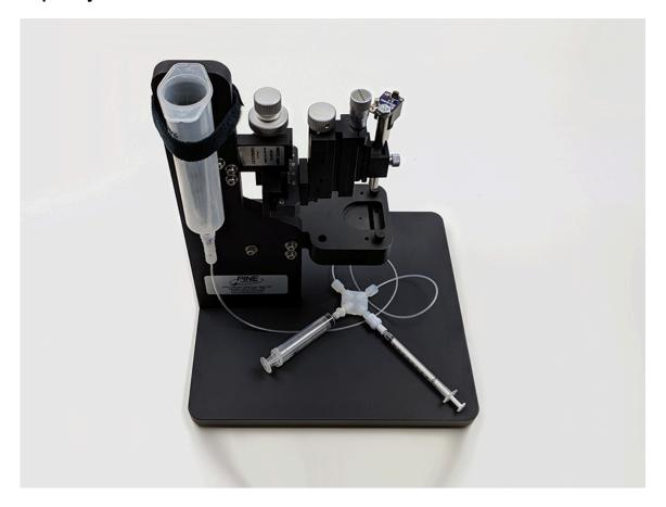
Figure 4-10. Fully Assembled Flow Cell
