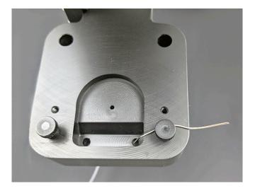
Figure 4-1. Reference Electrode Connection/Installation in Flow Cell
