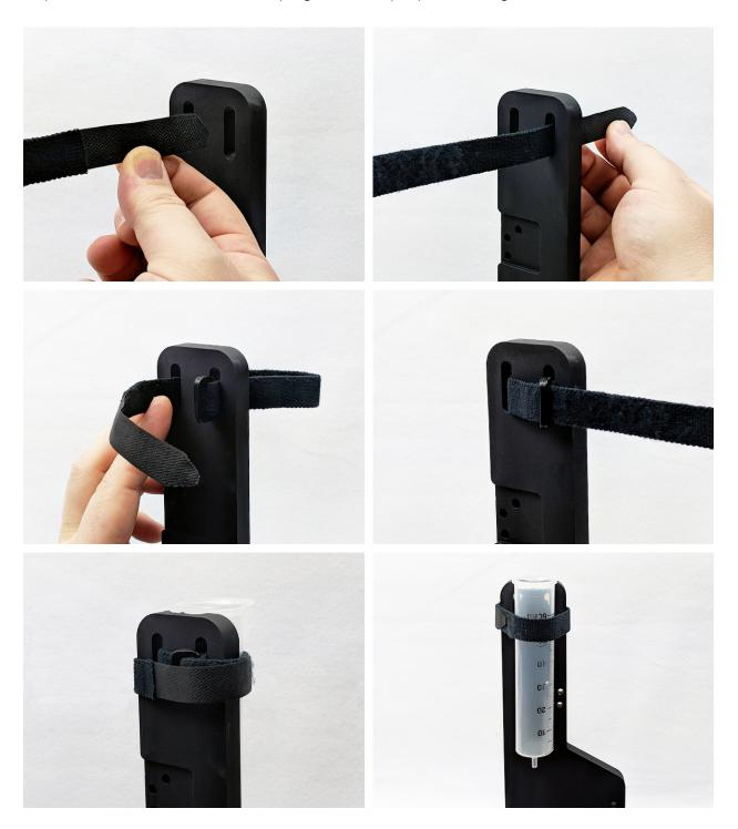
Figure 3-9. Attachment of Buffer Reservoir Strap (left to right, top to bottom)
