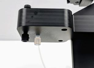
Figure 3-10. Flow Cell Delivery Line Connection to Flow Cell Body
