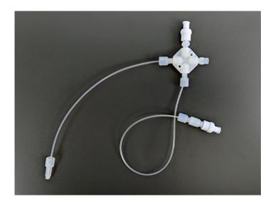
Figure 3-7. Fully Assembled Fluidics System
