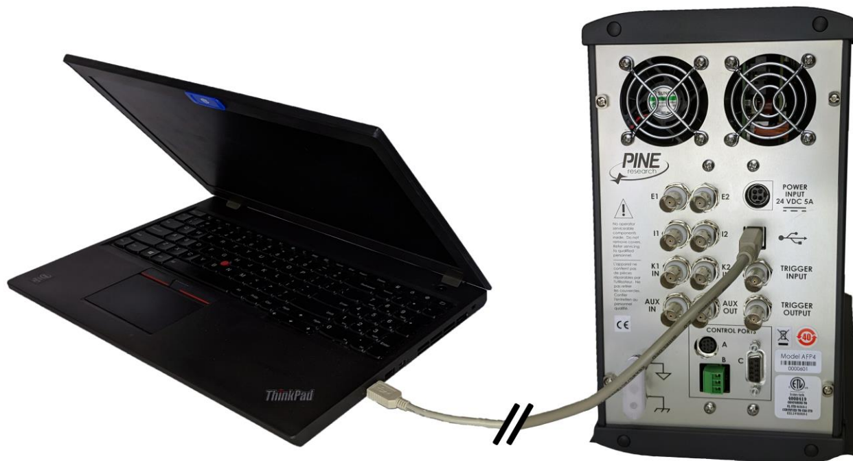
Figure 3-18. USB Cable Connection Between Potentiostat and Computer
