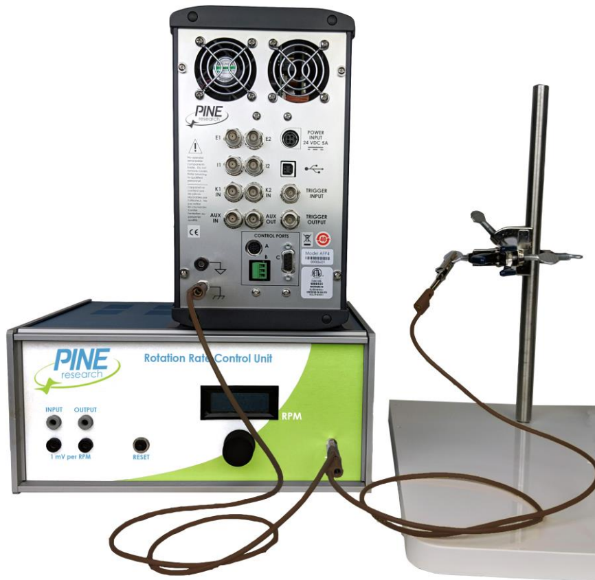
Figure 6-6. Connect All Instrument Chassis Terminals to a Common Point
