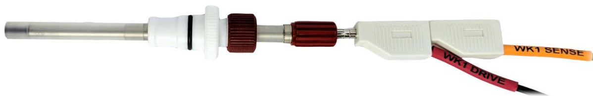
Figure 5-6. Working Electrode Sense and Drive Leads (K1) Shorted Together near the Electrode
