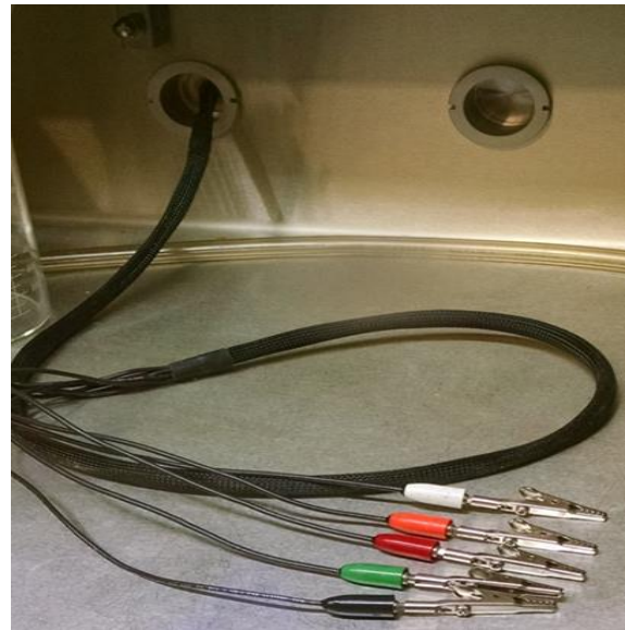
Figure 3-2. Cell Cable Glovebox Feedthrough
