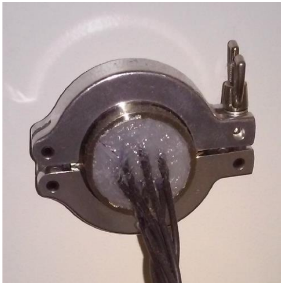
Figure 3-2. Cell Cable Glovebox Feedthrough
