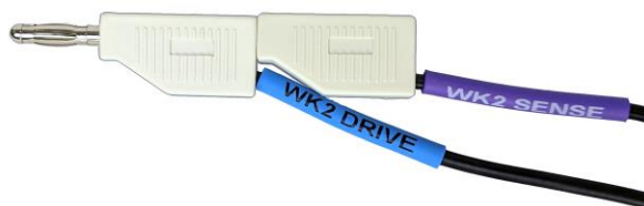
Figure 5-3. Unused K2 Electrode Lines
