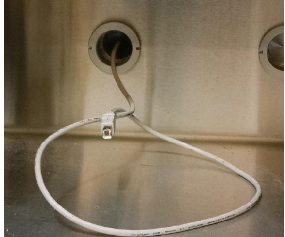
Figure 3-1. USB Cable Glovebox Feedthrough
