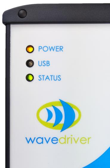
Figure 4-3. Indicator Lights on the Front Panel of the WaveDriver 40
