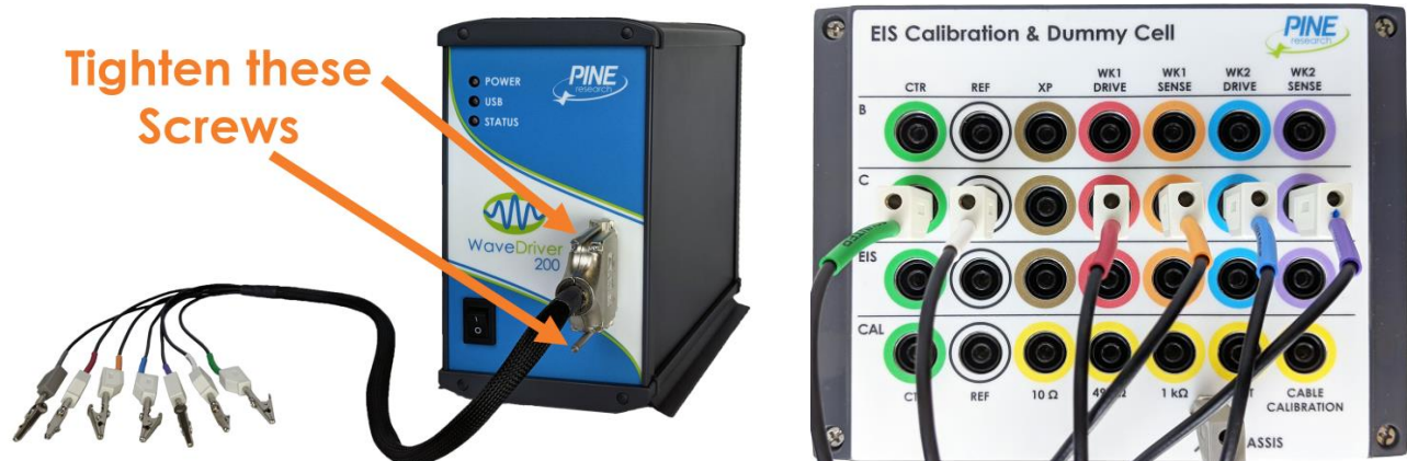
Figure 10-2. WaveDriver 200 Cell Cable Connected to Dummy Cell Row “C”
