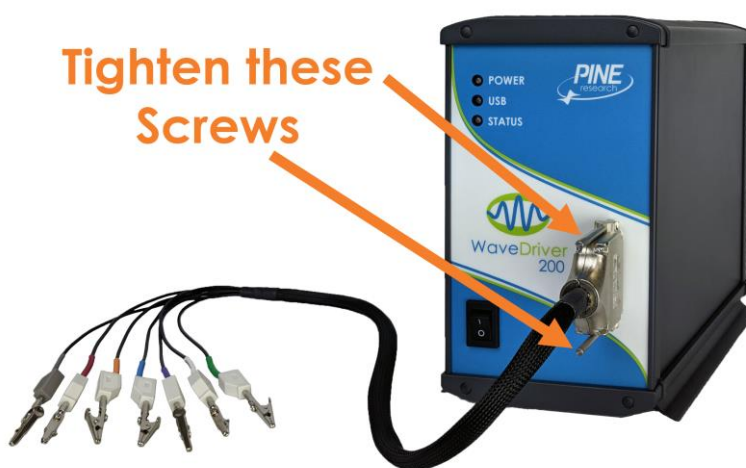
Figure 5-2. Secure Connection of the WaveDriver 200 Cell Cable to the Cell Port
