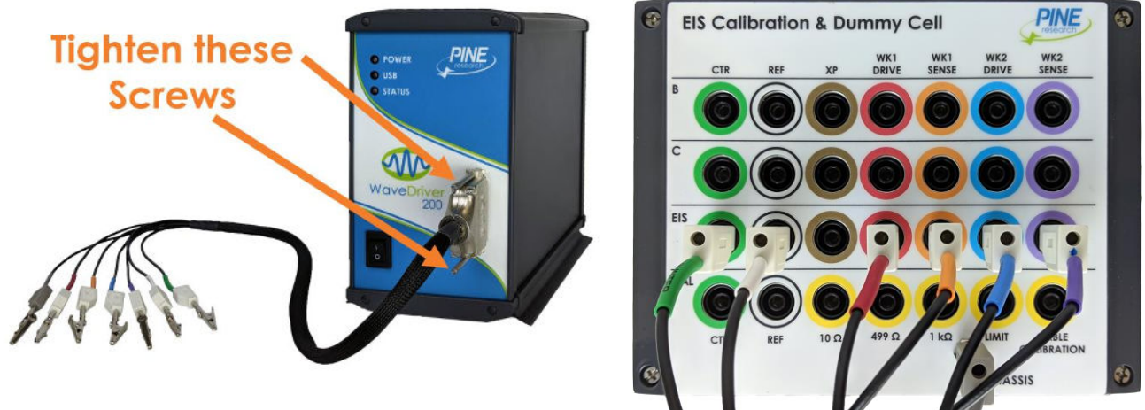
Figure 10-4. WaveDriver 200 Connections for a Simple EIS Test
