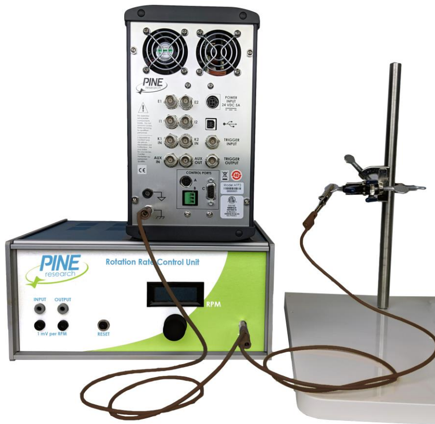
Figure 6-6. Connect All Instrument Chassis Terminals to a Common Point
