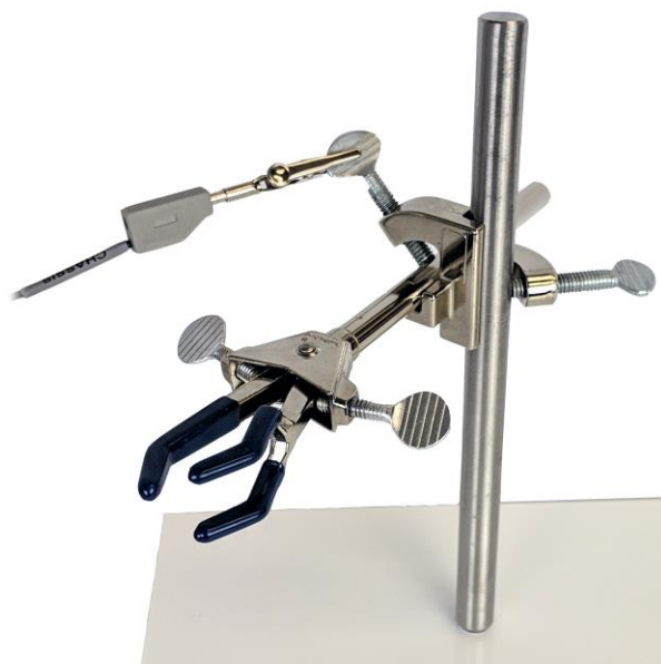
Figure 6-4. Metal Objects Near the Electrochemical Cell Should Be Grounded
