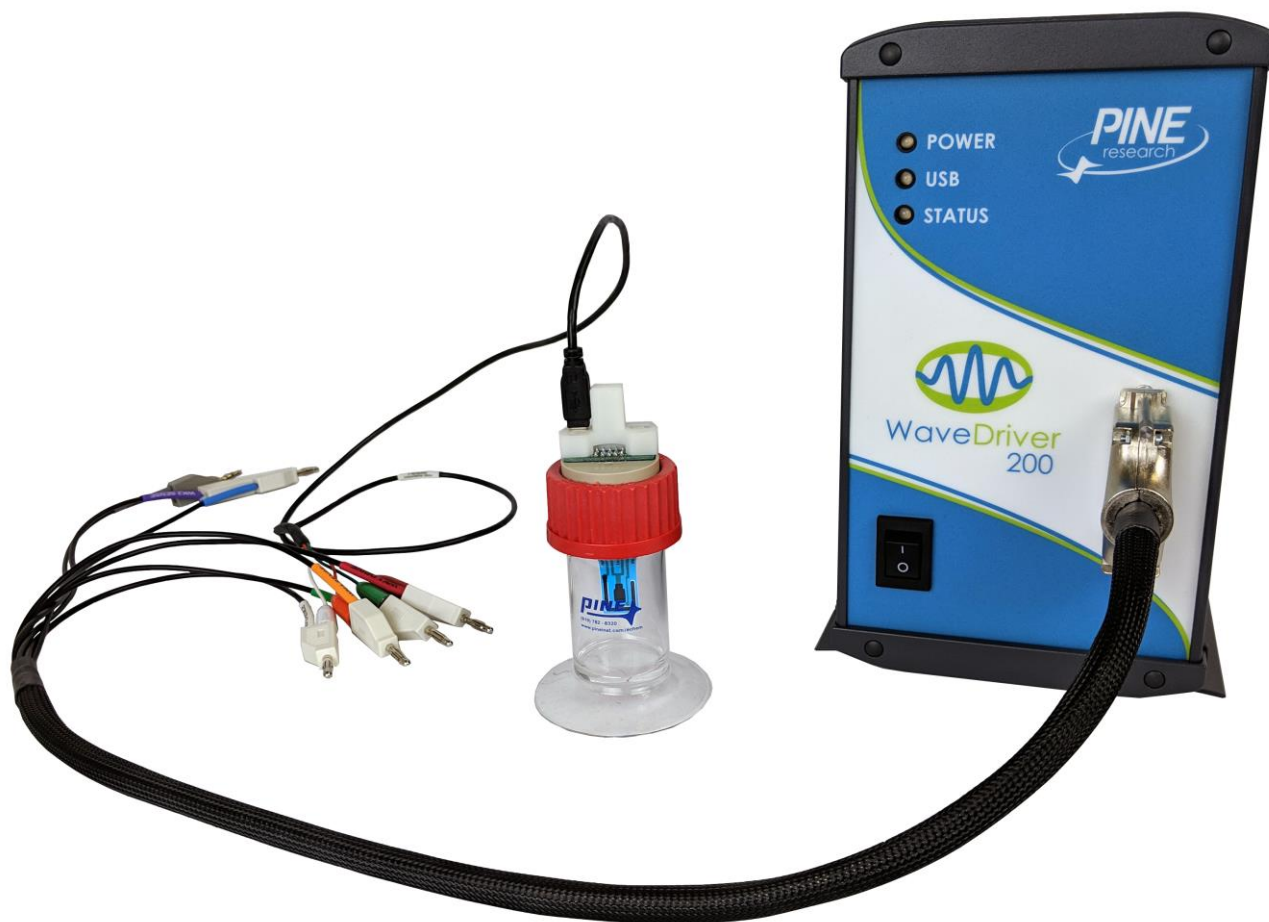
Figure 5-11. Cable Connections for the Compact Voltammetry Cell Kit
