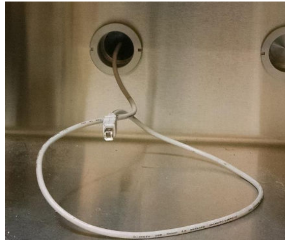
Figure 3-1. USB Cable Glovebox Feedthrough
