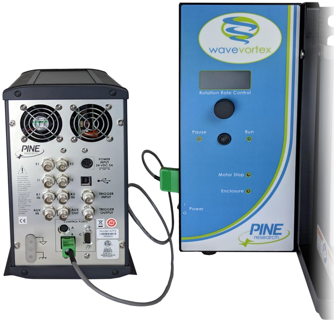
Figure 5-10. Rotation Rate Control Connections for a Pine Research WaveVortex 10 Rotator
