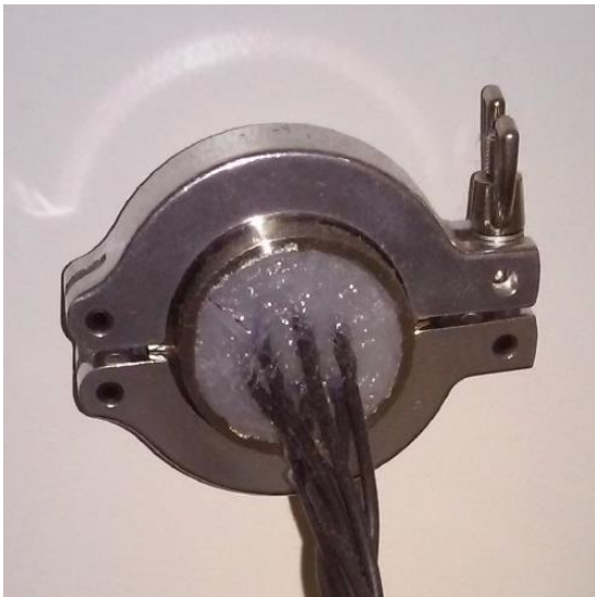
Figure 3-2. Cell Cable Glovebox Feedthrough
