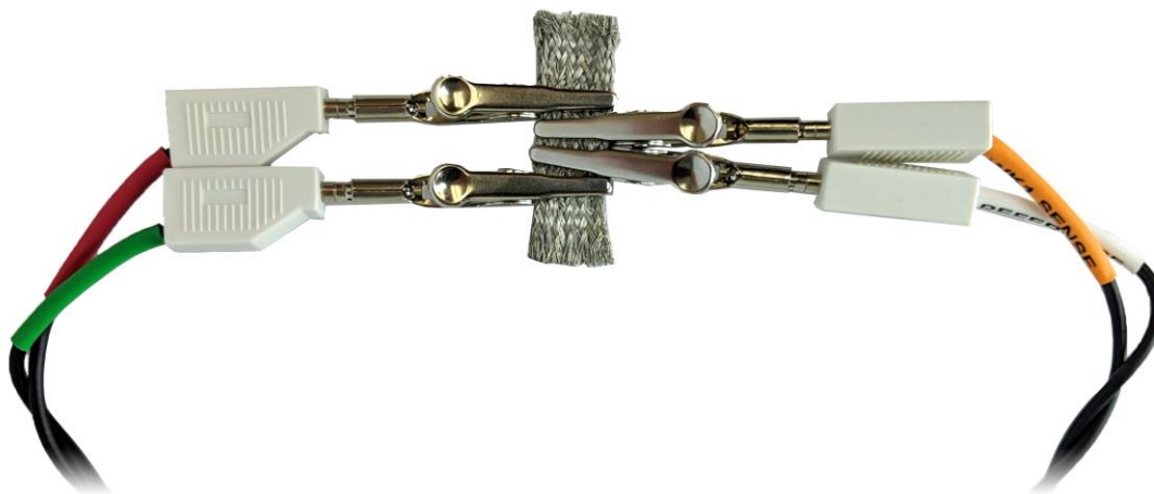
Figure 4-26. Braided Cell Cable Configuration for Low Inductance Load Measurement
