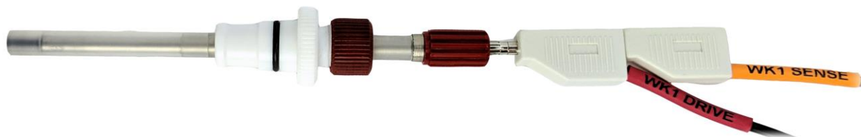
Figure 5-6. Working Electrode Sense and Drive Leads (K1) Shorted Together near the Electrode
