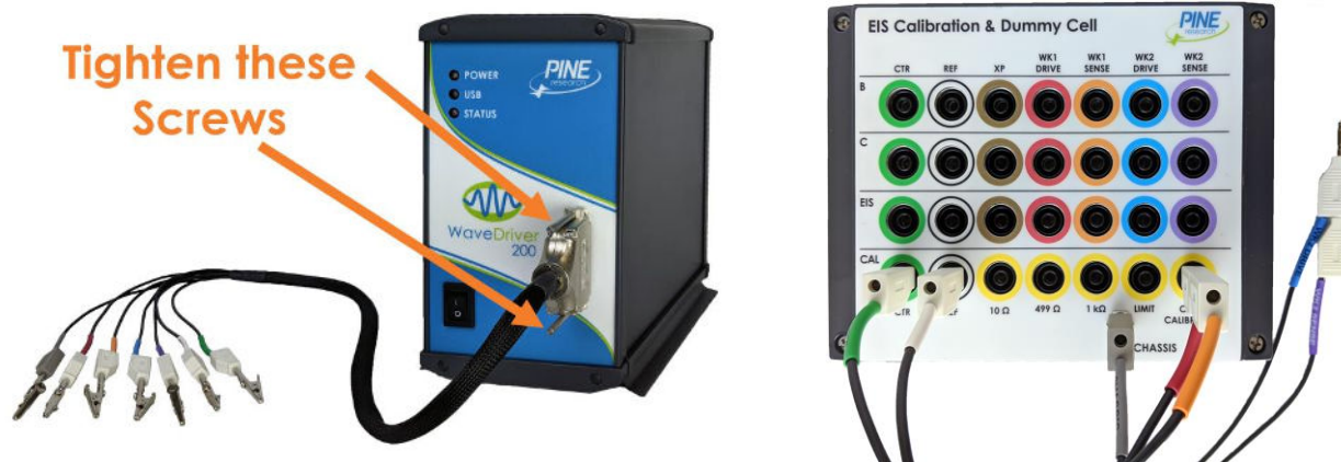
Figure 10-3. WaveDriver 200 Connections for Cell Cable Calibration
