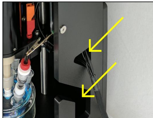
Figure 4-6. Access Slots for Cables and Tubing
