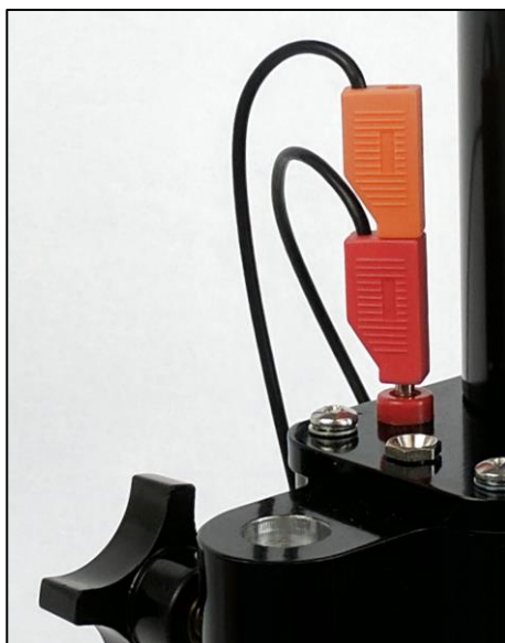
Figure 4-13. Electrode Connections for a Rotating Disk Electrode (RDE)
