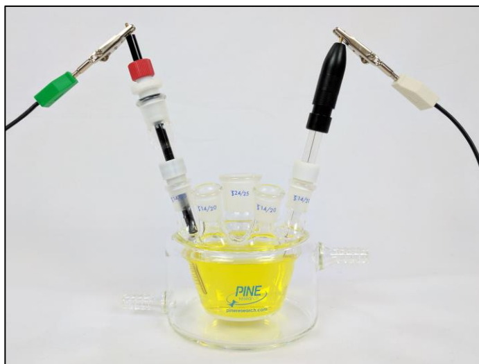
Figure 4-12. Connection of Counter and Reference Electrodes
