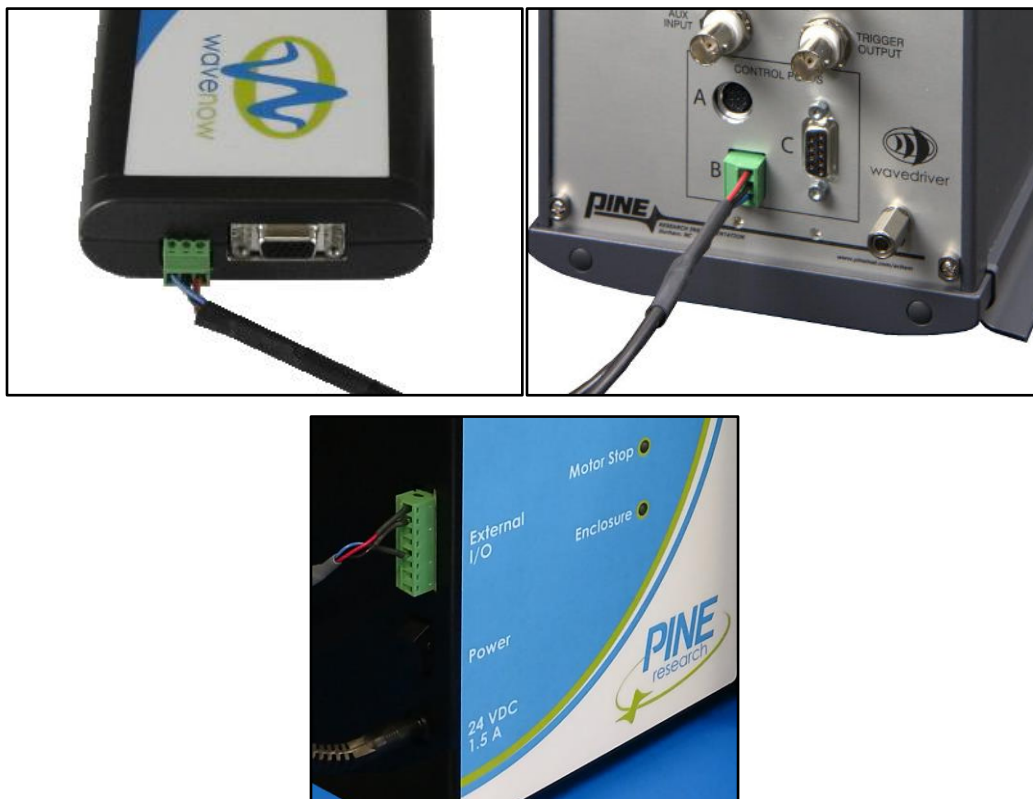
Figure 4-18. Connecting the Rotation Rate Control Cable
