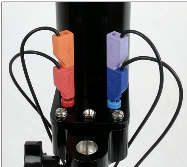
Figure 4-14. Electrode Connections for a Rotating Ring-Disk Electrode (RRDE)
