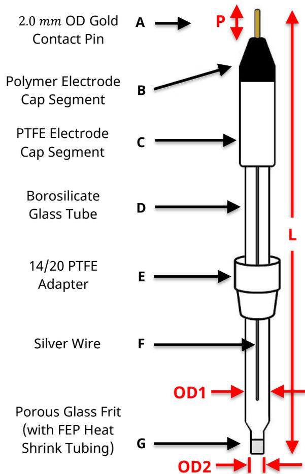
**Electrode Diameter (OD1):** 9.5 mm
