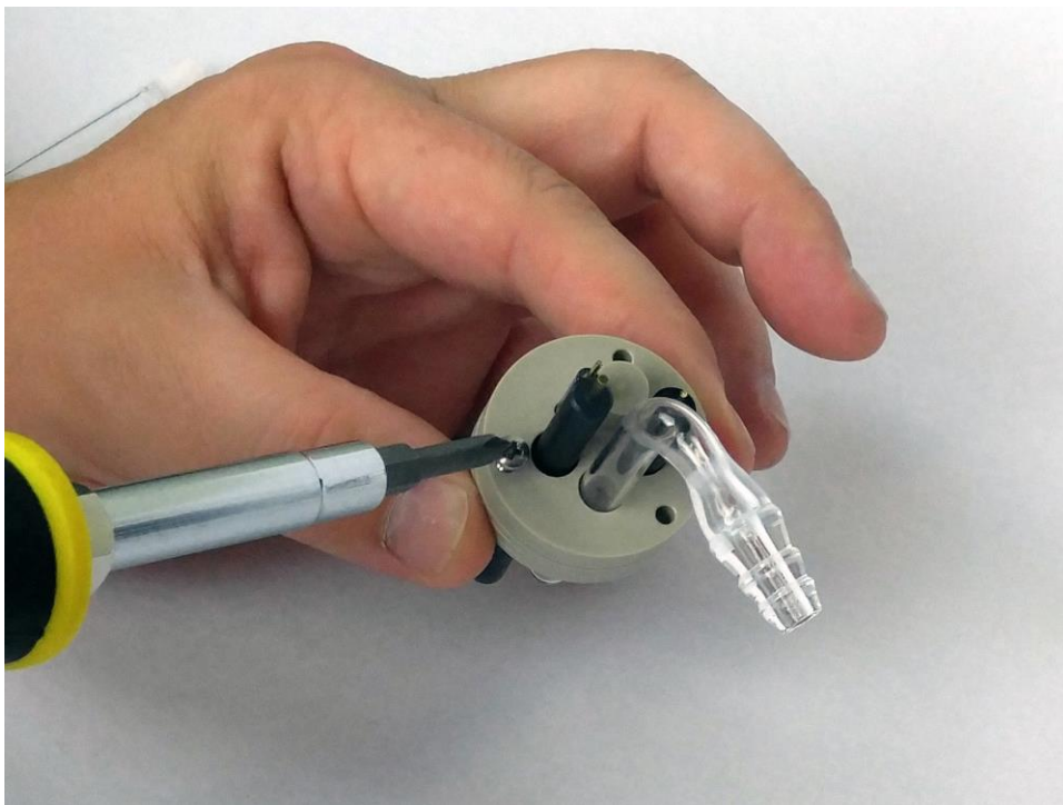
Figure 1-5. Install a screw to join the two cap halves. Loosely tighten one screw at a time to appropriately balance the cap seal. Note: DO NOT YET TIGHTEN SCREWS. It is useful to insert the cap kit with electrodes into the cell at this stage, before completely tightening the three screws. This allows any displaced air in the cell from becoming pressurized as the cap kit is pressed into place.
