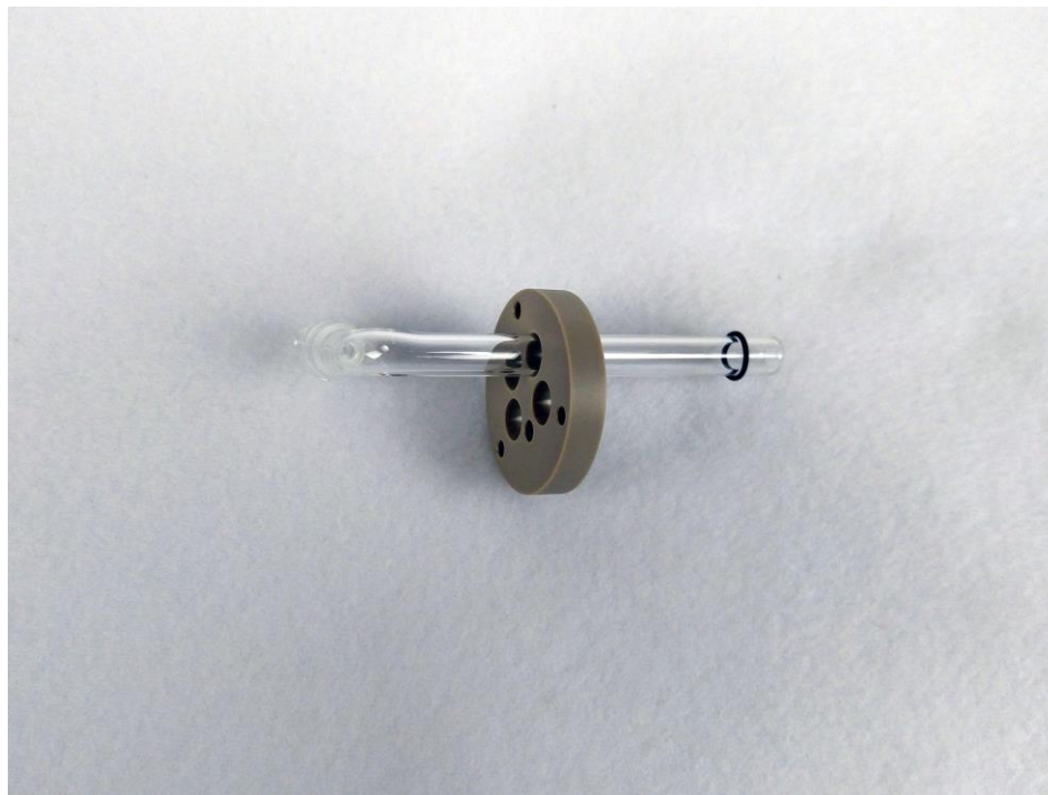
Figure 1-1. With the thin aspect of the cap kit, insert a probe (a purge tube in this image) through the appropriate hole and add an O-ring.
