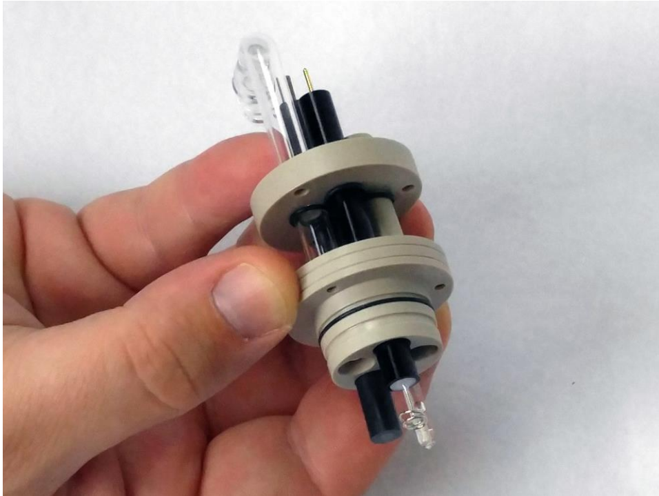
Figure 1-4. Slide the larger part of the cap kit onto the probes. Note: there is a directionality and the cap will only fit on in one orientation. Shown here is the cap kit with probes and O-rings installed, just before sealing the probes into the cap.
