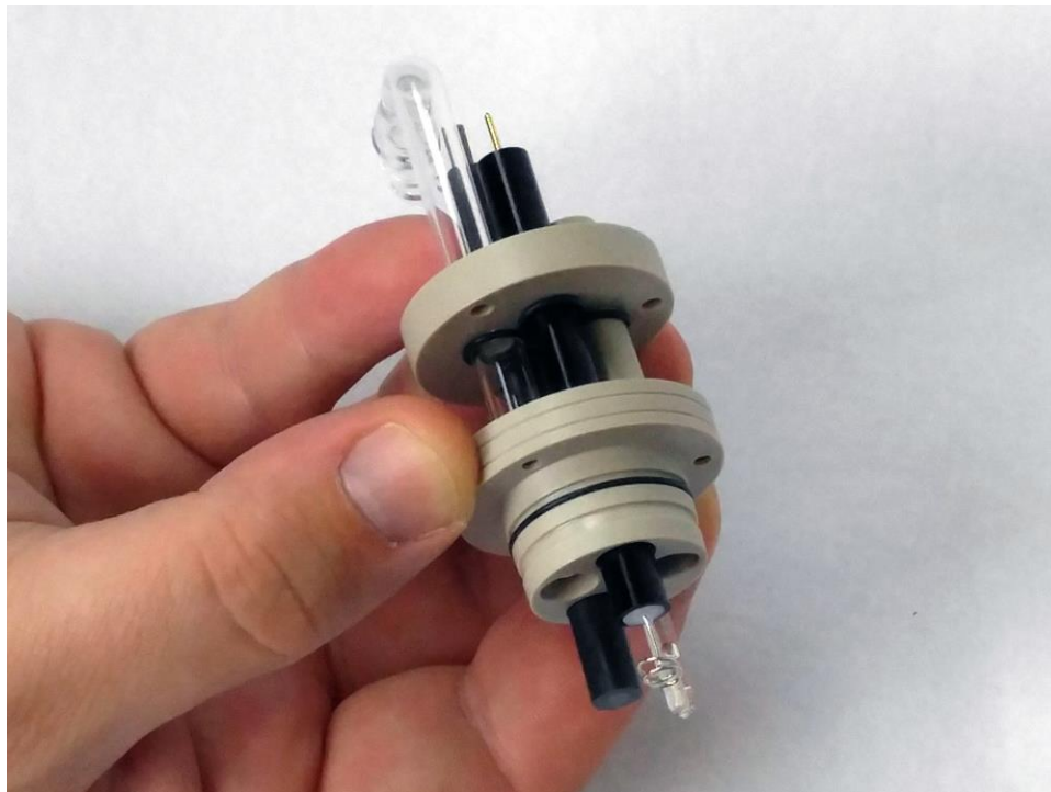
Figure 1-12. Slide the larger part of the cap kit onto the probes. Note: there is a directionality and the cap will only fit on in one orientation. Shown here is the cap kit with probes and O-rings installed, just before sealing the probes into the cap.
