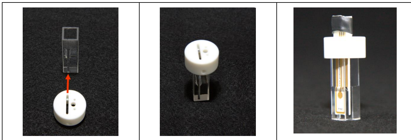
Figure 5-1. Proper Slot Alignment for the Quartz Cuvette, the Cap, and the Electrode Card
