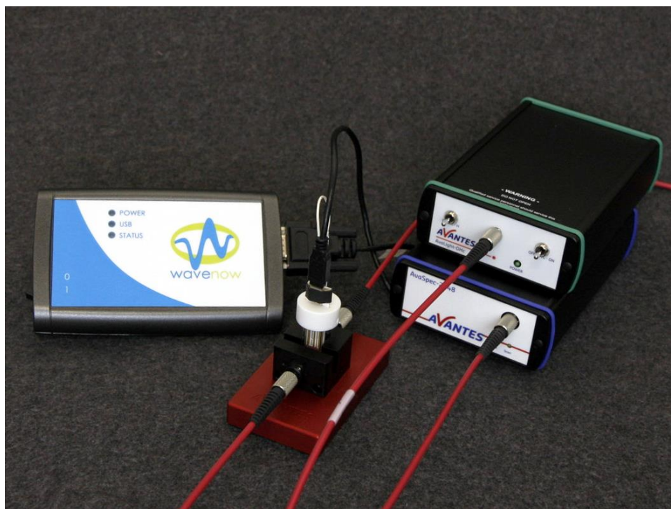
Figure 5-9. Light Source Must Illuminate the Electrode Card on the Side with the Metal Electrodes
