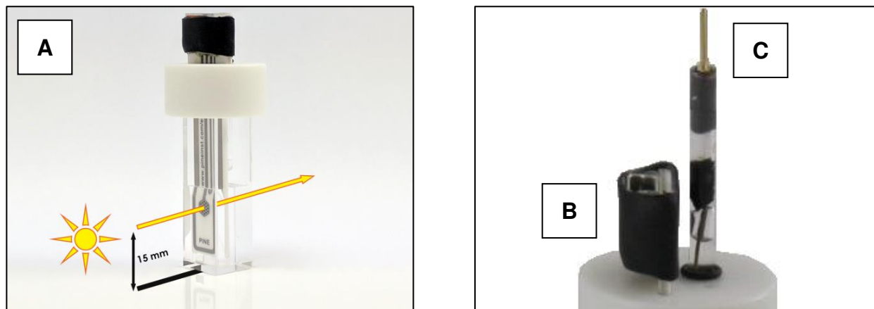
Figure 2-1. Beam Path and Electrical Connections for the Honeycomb Electrode
