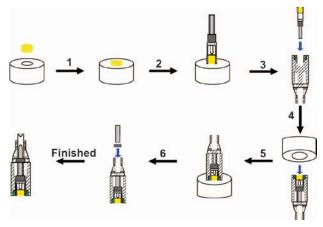
1. Set the mounting block on a flat surface with the small bore facing upwards. Carefully drop the disk insert into the mounting block. The polished surface of the disk insert should face downwards. The disk insert should be centered and should rest in a shallow well located within the small bore.
