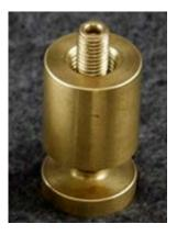
To eject the disk insert, remove the disk core nut from the electrode tip and invert the electrode tip so that the disk core washer falls out.
