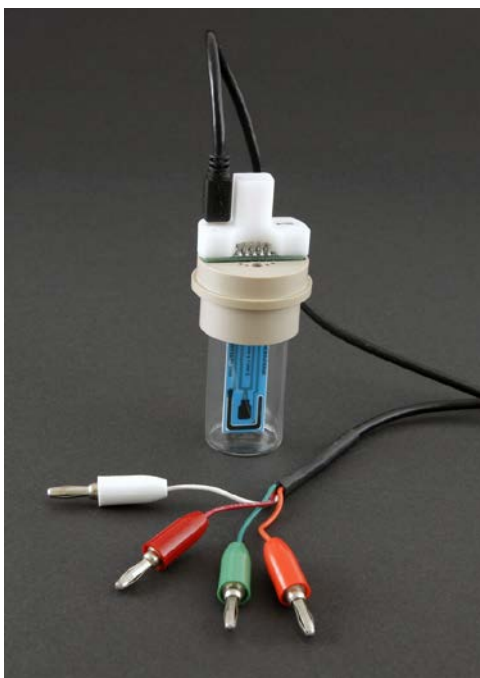
Figure 4. Connecting the Generic Cable to the Compact Voltammetry Cell
