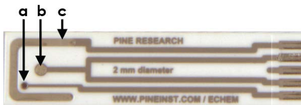
Figure 11. a) Reference Electrode, b) Working Electrode, and c) Counter Electrode for a Ceramic SPE
