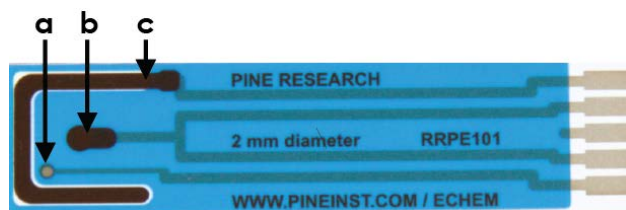
Figure 2. a) Reference Electrode, b) Working Electrode, and c) Counter Electrode for a SPCE
