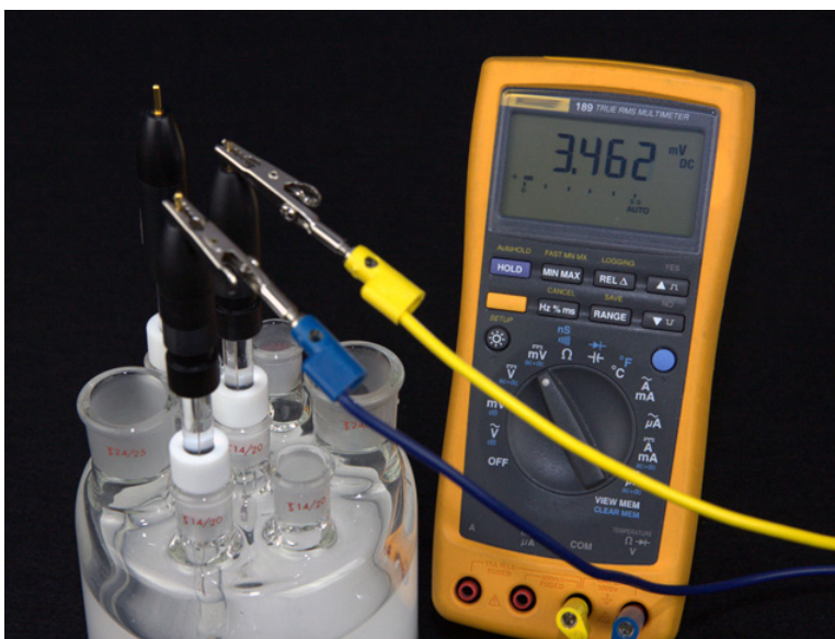
Figure 4. Reference Electrode Test with a Multimeter
