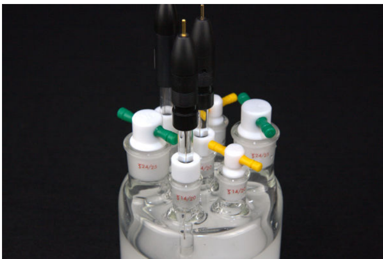
Figure 3. Example Reference Electrode Storage Container with Proper Sealing
