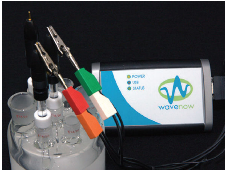
Figure 5. Reference Electrode Test with a Potentiostat
