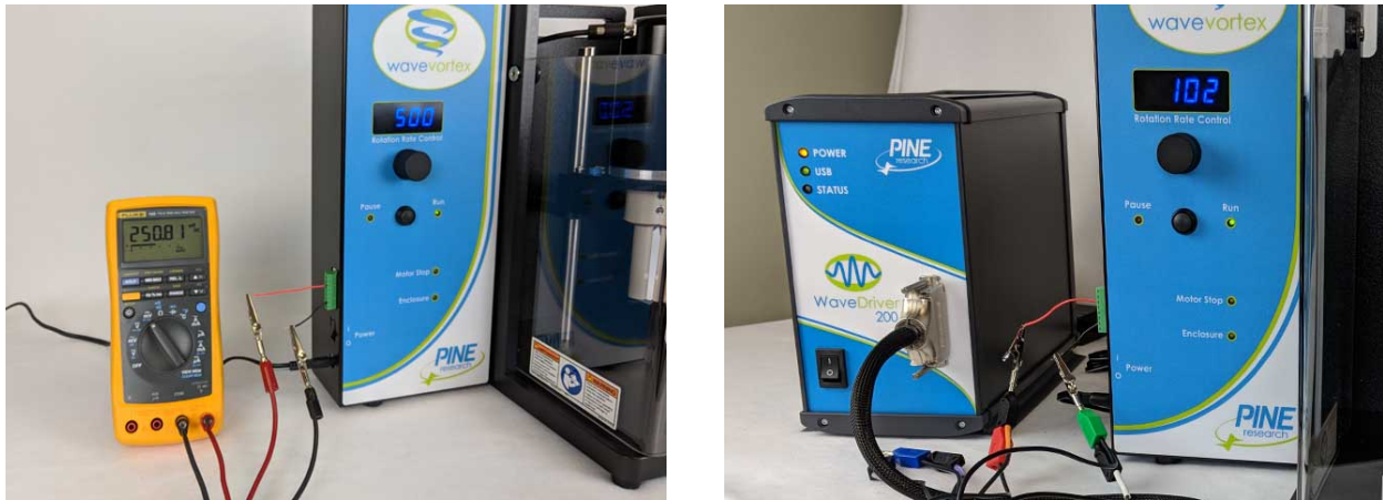
Figure 3-3. Calibration Verification by Measuring Output Voltage with a Voltmeter (Left) and Potentiostat (Right)
