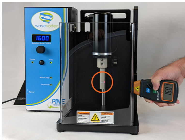
Figure 2-6. Positioning of the Handheld Tachometer and its Beam Hitting the Rotating Shaft
