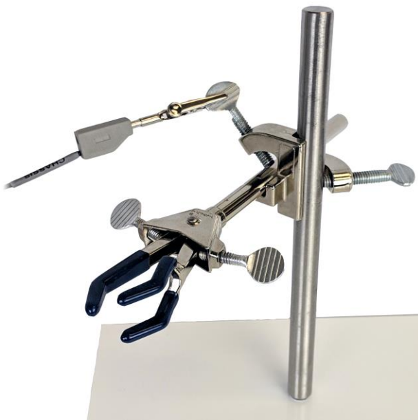
Figure 4-17. Metal Objects Near the Electrochemical Cell Can be Grounded
