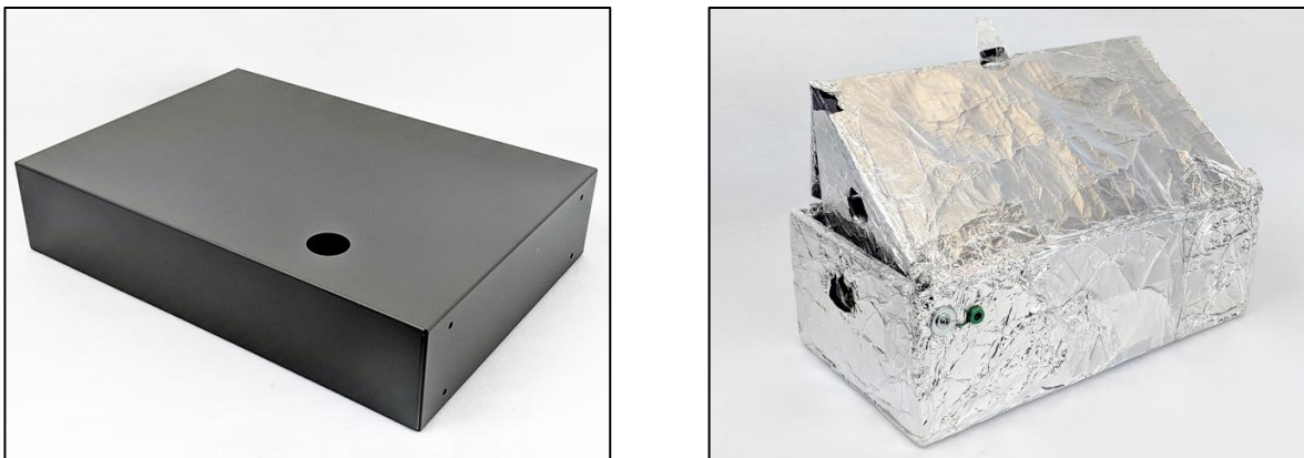
Figure 4-16. Common Examples of Faraday Cages
