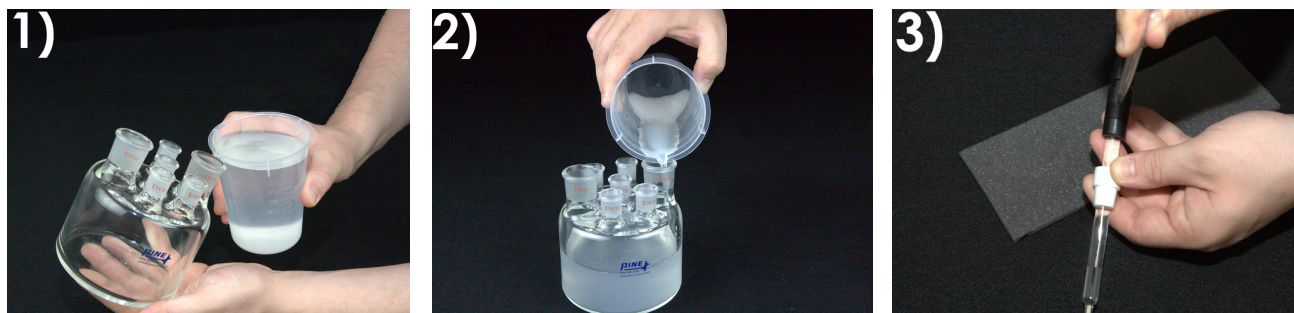
Figure 2. Steps to Prepare a Master Reference Electrode and Storage Cell
