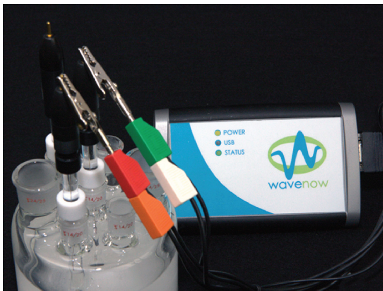
Figure 5. Reference Electrode Test with a Potentiostat
