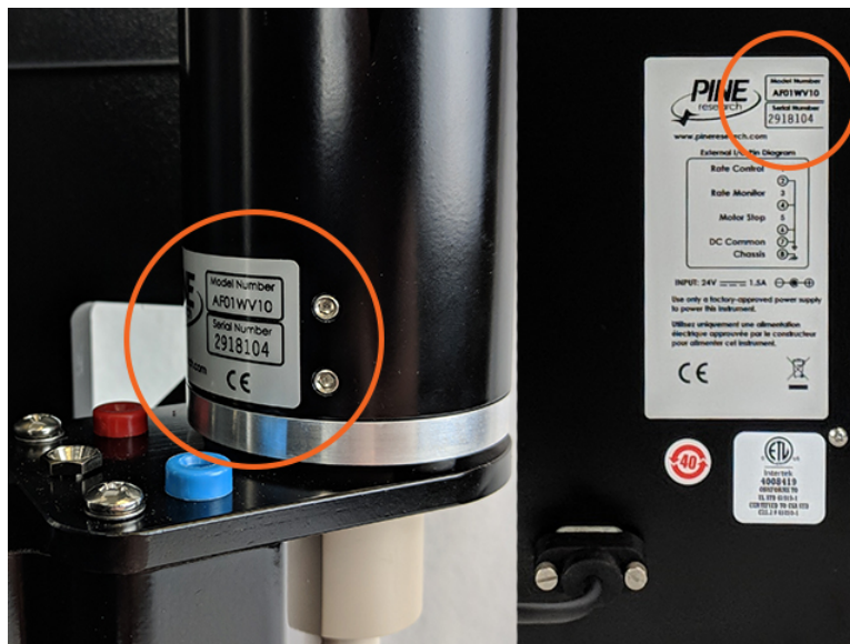
Figure 2-1. Motor Head and Control Unit Labels with Serial Numbers Circled
