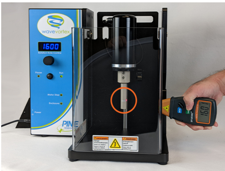
Figure 2-6. Positioning of the Handheld Tachometer and its Beam Hitting the Rotating Shaft
