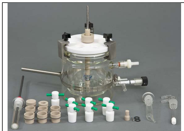
Figure 7-1. Components of the 15 mm OD RCE System.
