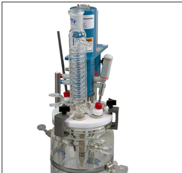
Figure 1-1. Fully Assembled Pine Research Instrumentation 15 mm OD Rotating Cylinder Electrode System.
