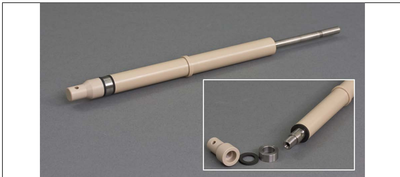
Figure 9-1. Assembled and Disassembled Views of the 15 mm OD Rotating Cylinder Electrode.
